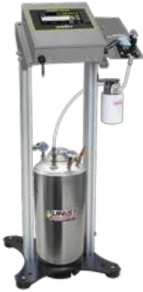
The 4 gallon [15 liter] stainless steel pressure tank comes equipped with a 0-100 psi [0-7 bar] regulator and a low level switch.
