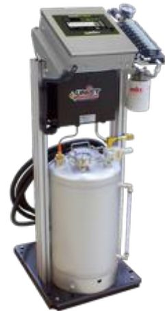
The auto refill fluid supply system incorporates a 10 gallon [38 liter] ASME rated stainless steel pressure tank with 0-60 psi [0-4 bar] precision regulator and integral high and low level switches. The system also includes PLC controls and an electric pump to automatically refill the tank, which eliminates down time. This system provides superior performance when drawing fluid from a tote or drum.
